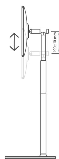
A side view of the TV on its stand. A vertical double-headed arrow indicates the height of the stand is adjustable. A dimension line next to the arrow shows the range is $190 \pm 10$ mm. |
